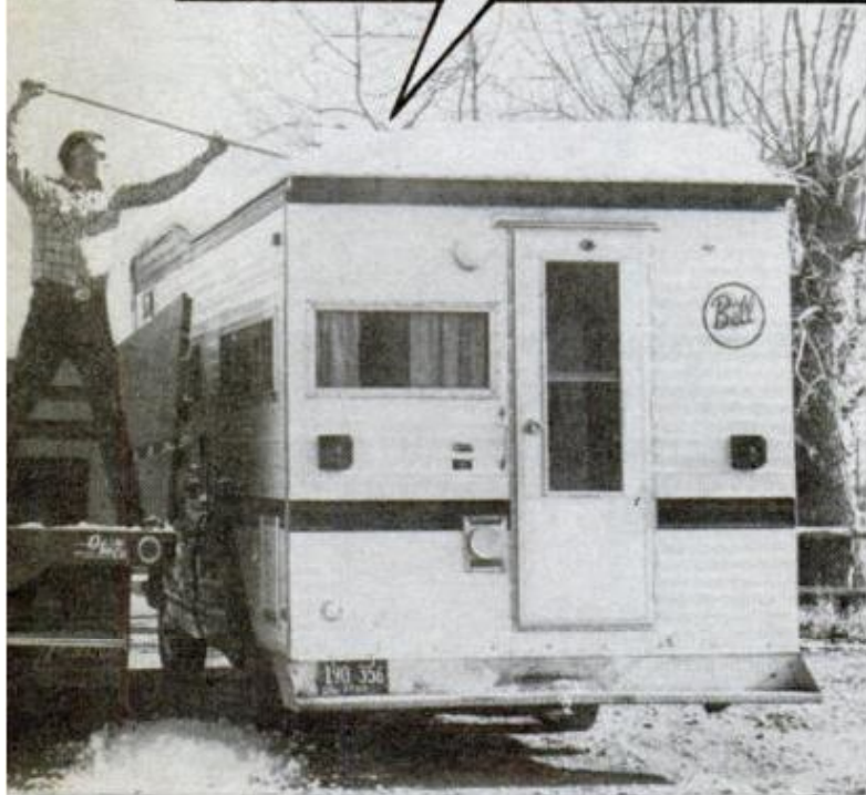
ONE DANGER OF WINTER CAMPING is a snow-blocked vent (above). Check all camper vents regularly before cooking, heating or going to bed, and keep the coach roof free of heavy accumulations of snow
